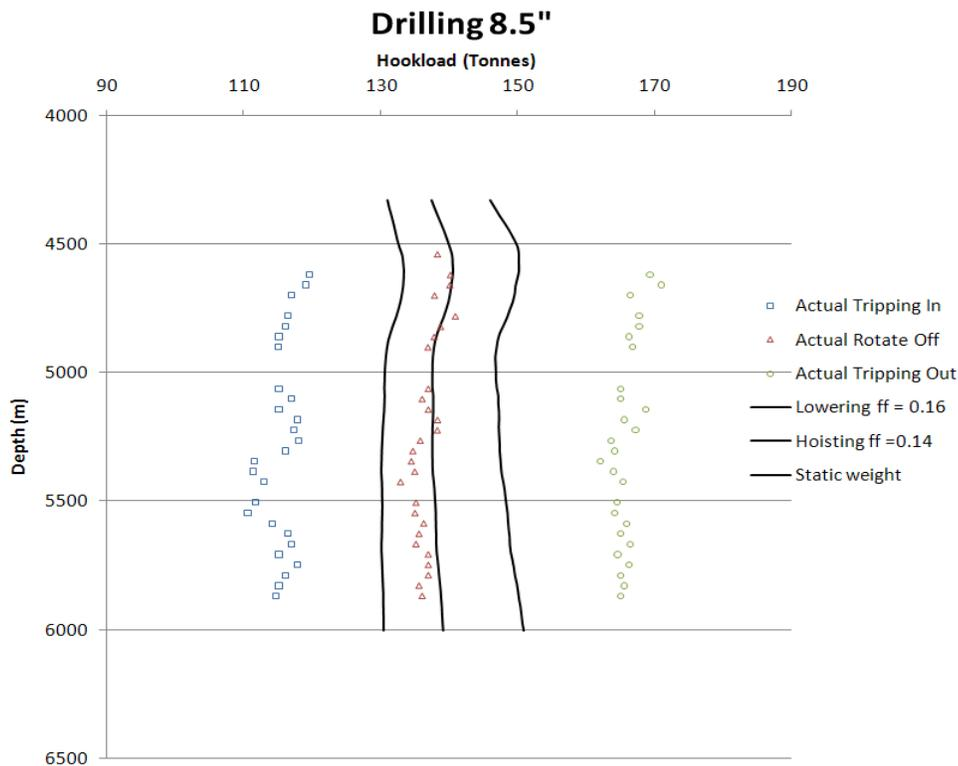
**Figure 9: Sheave friction correction applied to the model.**
