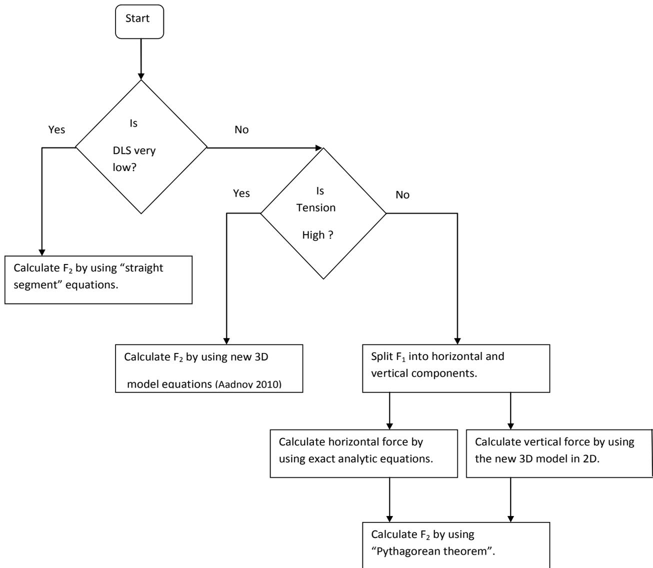
**Figure 5: Flow diagram showing how to calculate tension on top of a segment**
