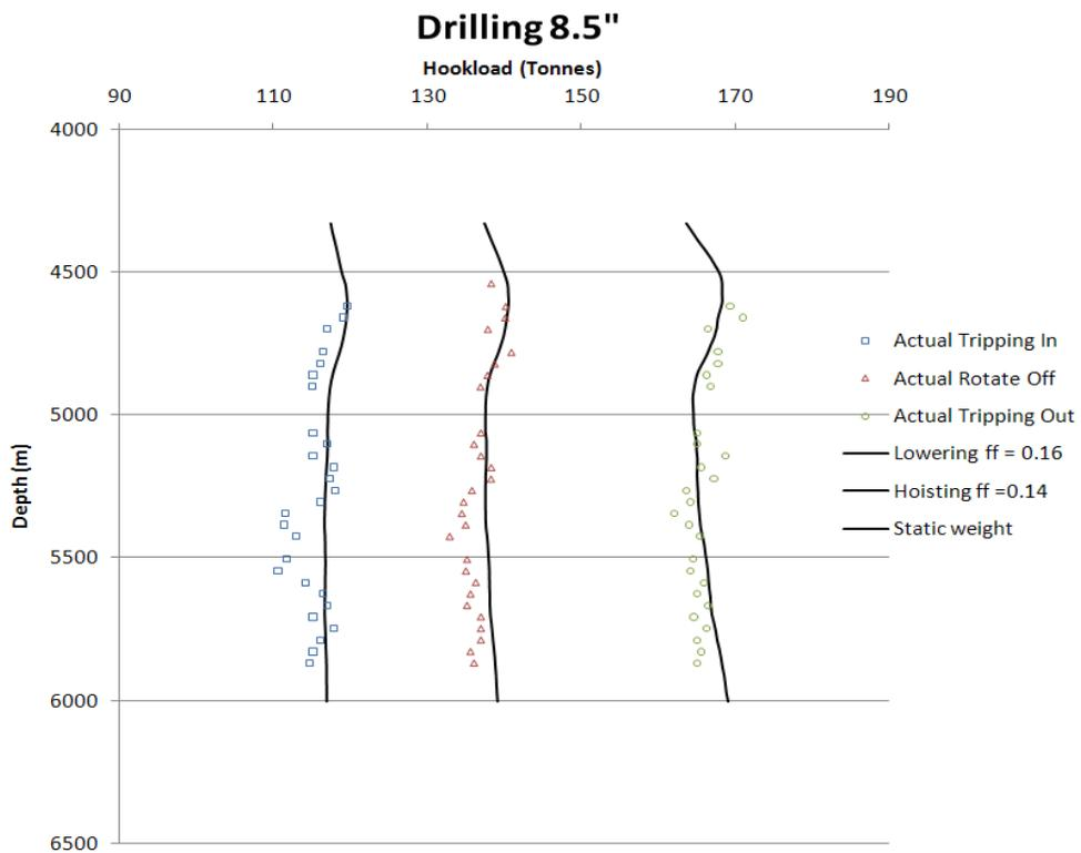
Figure 8: Matching actual data with no sheave friction correction.
