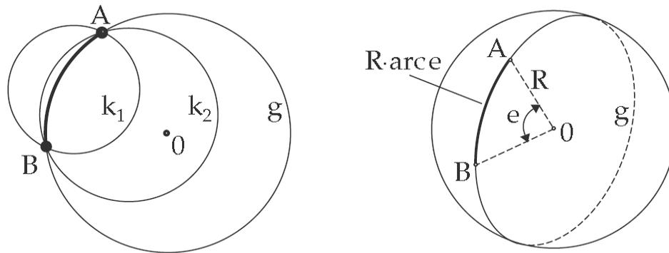
**Figure 4: Minimum curvature method**
