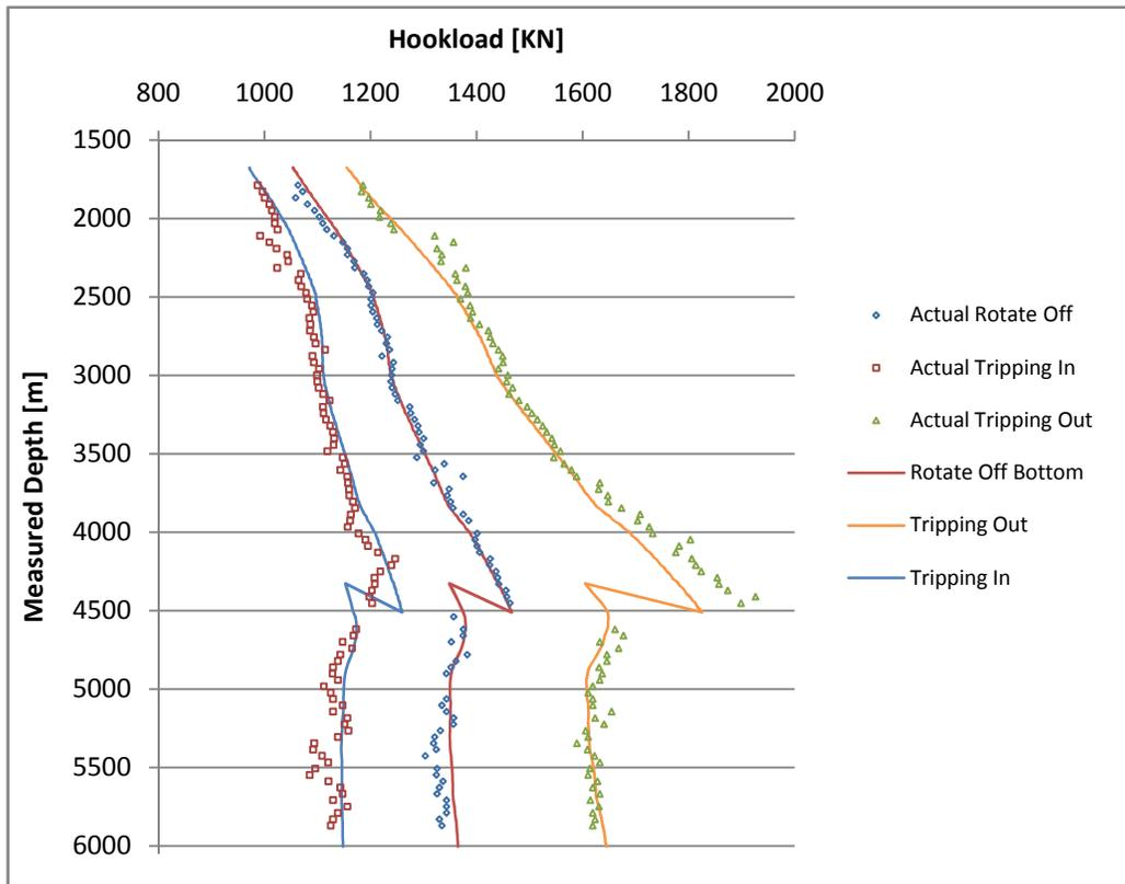
Figure 7: From Wellplan, drilling 12.25" and 8.5"
