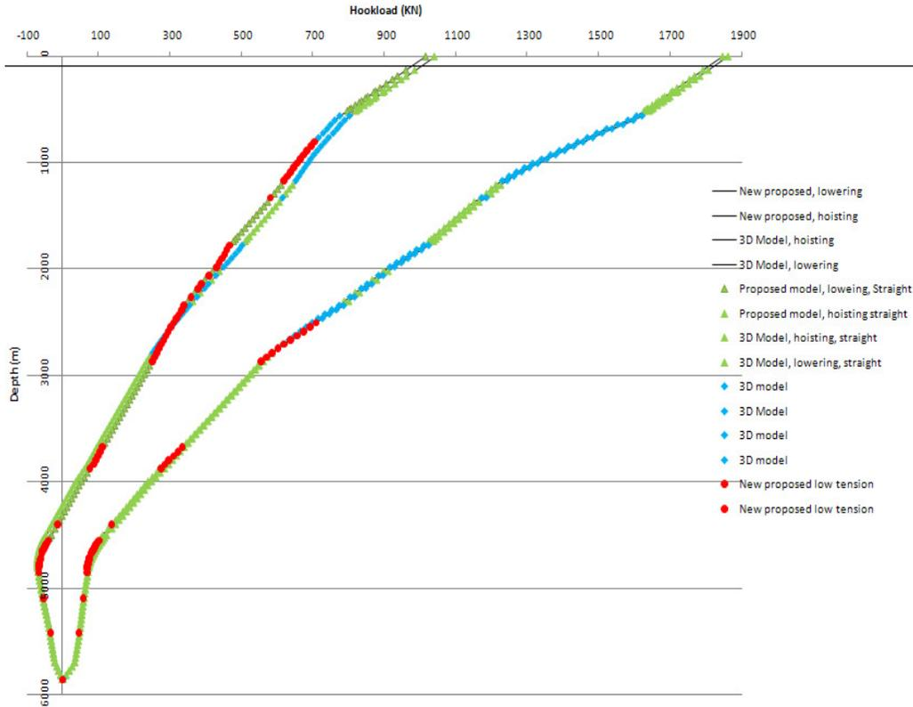
Figure 12: Hoisting and lowering with the new model
