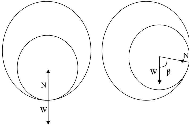
Figure 2: Forces due to gravity on horizontal pipe
