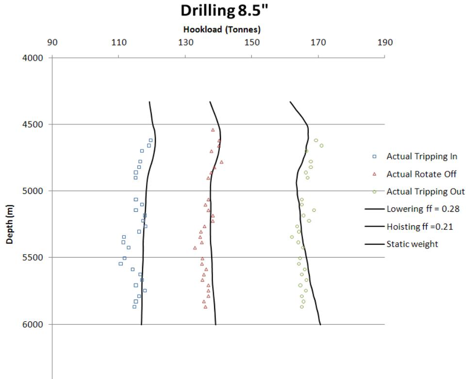
**Figure 10: Matching the actual data with sheave friction correction and higher more realistic friction factors**
